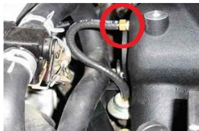
Figure 5: Boost Reference Source (Backside of Supercharger)
